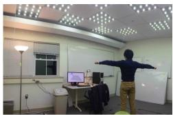
The StarLight system is designed to track a person's behaviour and reconstruct 3D skeleton regardless of furniture obstruction. The technology can be applied to various aspects, such as virtual reality and health monitoring. You may find more information from the <u>StarLight</u> webpage.
