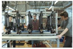
Project Escher is an innovative 3D printing system that integrates simultaneous and parallel printing of several 3D printers to fabricate a complex large scale product. Visit the <a href="Project Escher">Project Escher</a> website to discover more.
